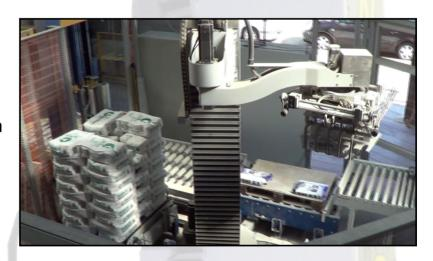
The new palletizer works in unison with both production lines, palletizing both the paper valve bags and the polyethylene bags, simultaneously if necessary.
